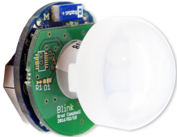
Figure 6.5: Blink sensor used for occupancy sensing. This passive infrared (PIR) sensor can be added to the existing energy metering system to correlate device activity with occupancy. The sensor gives a binary occupancy indication, and operates on a similar wireless protocol to PowerBlade and BLEES. Periodically Blink sends new occupancy data in a BLE advertisement packet.
