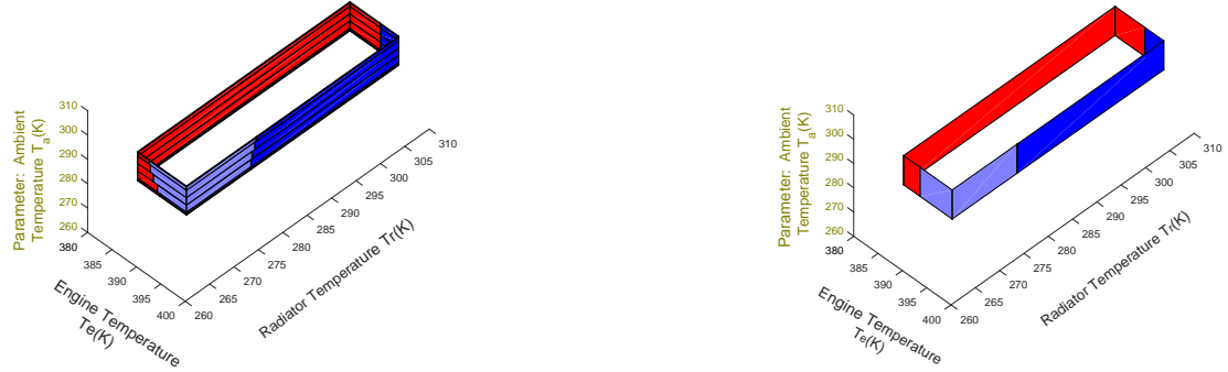
Fig. 3. Example 2: parametrized (left) and robustified (right) controller. Red: u = 1 , light blue: u = 3 , dark blue: u = 4 .
