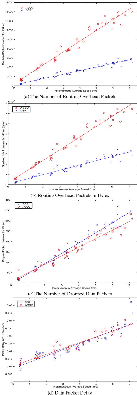
Fig. 6. Performance Metric vs. Instantaneous Average Node Speed
