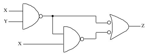
Assume that each gate has 1 unit of delay. (Delay time = 1 on timing diagram.) Draw the output waveform (Z) for the given input values of X & Y.
