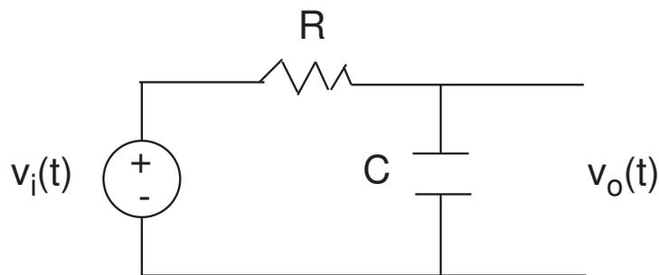
Input: applied voltage, Output: voltage across capacitor
