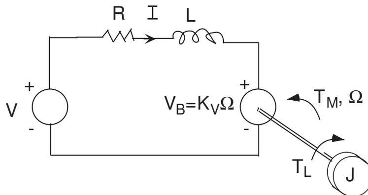
Input: applied voltage, Output: current, torque, speed
