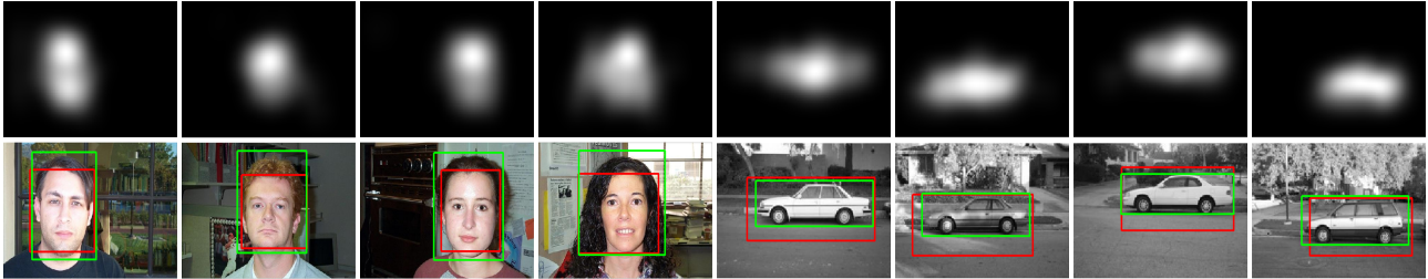
Figure 4. Visualization of (top) the switch unit activation map and (bottom) the images overlaid with the predicted (red) and the ground truth bounding boxes (green).
