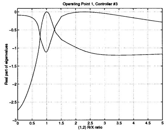
Fig. 5: Controller 3, Real part of compensated system eigenvalues
