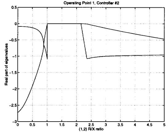
Fig. 4: Controller 2, Real part of compensated system eigenvalues
