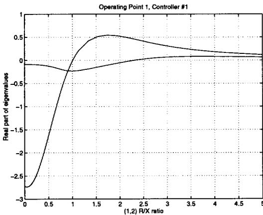
Fig. 3: Controller 1, Real part of compensated system eigenvalues
