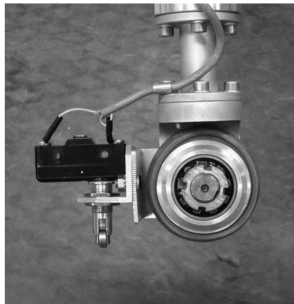
Figure 6.5: RABBIT's frontal plane leg end wheel with contact switch.
