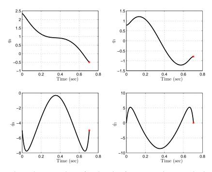
Fig. 14. The computed open-loop control transfers the robot from its initial state to the desired final state (\*).
