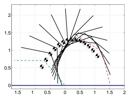
Fig. 12. The motion of the robot passes from left to right, with a singular position occurring when the two links are aligned. The initial configuration  $(\cdot - \cdot - \text{green})$  and final configuration  $(\cdot - \cdot - \text{red})$  belong to different configuration classes.
