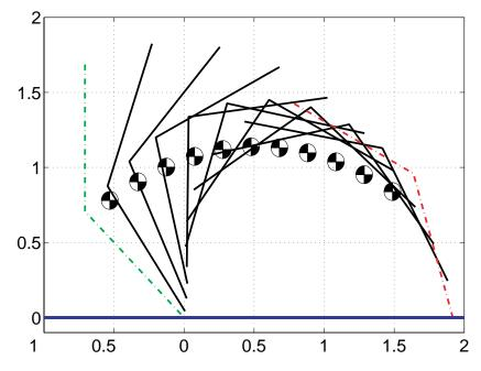
Fig. 9. The motion of the robot passes from left to right without passing through a singularity. The initial configuration  $(\cdot - \cdot - \text{ green})$  and final configuration  $(\cdot - \cdot - \text{ red})$  belong to the same configuration class. The center of gravity follows a parabolic trajectory.
