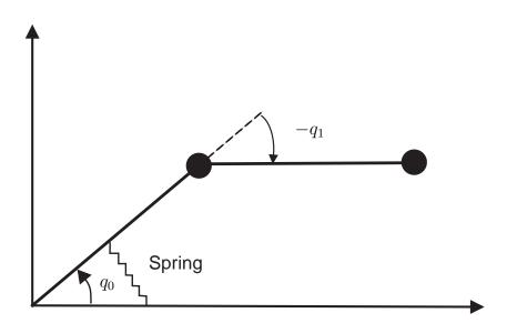
Fig. 3. A two-link robot attached to a pivot and constrained to move in a horizontal plane. The joint  $q_1$  is actuated, while  $q_0$  is passive; a linear spring with stiffness  $K_s$  is attached with rest position  $q_0 = 0$ . From left to right, the links have length  $L_1$  and  $L_2$  and the masses are  $m_1$ ,  $m_2$ .
