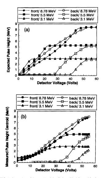
FIG. 4. Comparison of front and back irradiation with alpha particles for a 45- $\mu$ m-thick bulk GaAs detector. Shown are (a) the numerically calculated pulse height responses and (b) the measured pulse height responses. The alpha particle energies are 3.1, 5.5, and 8.78 MeV.  $\mathcal{E}_c$  is  $7.0 \times 10^3$  V/cm and  $\alpha$  is 15. The pulse height response is shown in terms of energy (MeV) measured from the detector.
