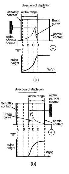
FIG. 2. Expected voltage dependent pulse height responses to alpha particles from an extrinsic Schottky barrier diode detector. Depicted are the (a) expected pulse height response due to front side irradiation (Schottky contact) and (b) the expected pulse height response due to backside irradiation (ohmic contact). Notice that pulses will be observed at low voltages for front side irradiation, however pulses will not be observed from backside irradiation until a threshold voltage is reached.
