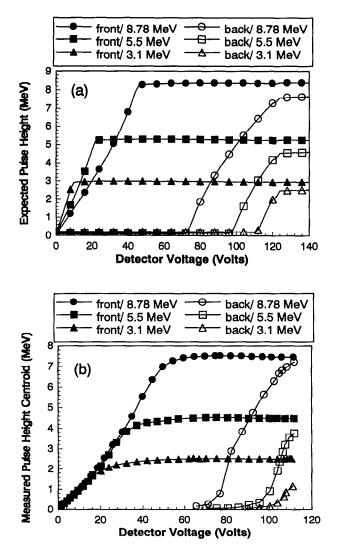
FIG. 5. Comparison of front and back irradiation with alpha particles for a 100- $\mu$ m-thick bulk GaAs detector. Shown are (a) the numerically calculated pulse height responses and (b) the measured pulse height responses. The alpha particle energies are 3.1, 5.5, and 8.78 Mev.  $Z_c$  is  $7.0 \times 10^3$  V/cm and  $\alpha$  is 15. The pulse height response is shown in terms of energy (MeV) measured from the detector.
