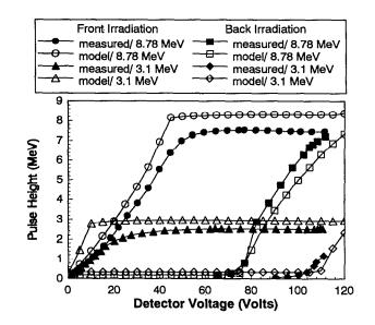
FIG. 7. Overlay comparison between modeled and measured pulse height curves for a 100- $\mu$ m-thick bulk GaAs detector. Shown are the curves for 3.1 and 8.78 MeV alpha particles where the pulse height response is shown in terms of MeV.  $\mathcal{K}_c$  is 7.0×10<sup>3</sup> V/cm and  $\alpha$  is 15 for the modeled pulse height curves.
