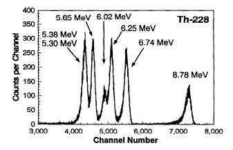
FIG. 6. Alpha particle differential pulse height spectrum from <sup>228</sup>Th taken with a 100  $\mu$ m bulk GaAs detector. The detector was irradiated in vacuum from the front contact (Schottky contact).
